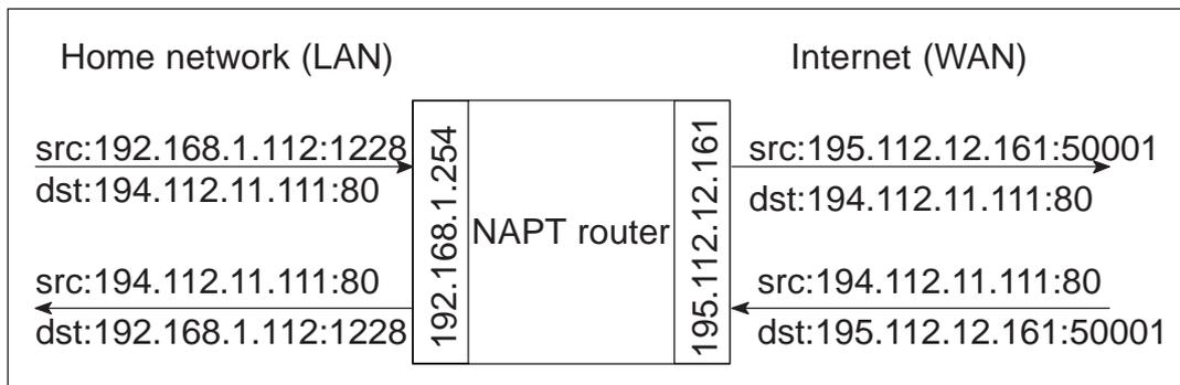
**Figure 19** Principle of Network Address Port Translation
